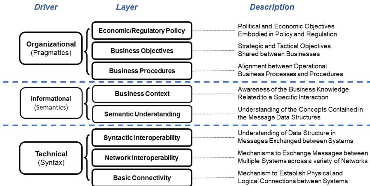
**Figure 10.** The GridWise Architecture Council’s interoperability framework (GWAC 2008)
