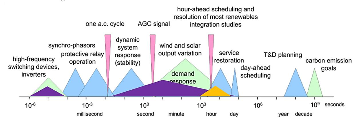
**Figure 3.** Electric power system timelines (von Meier 2012; used with permission).
