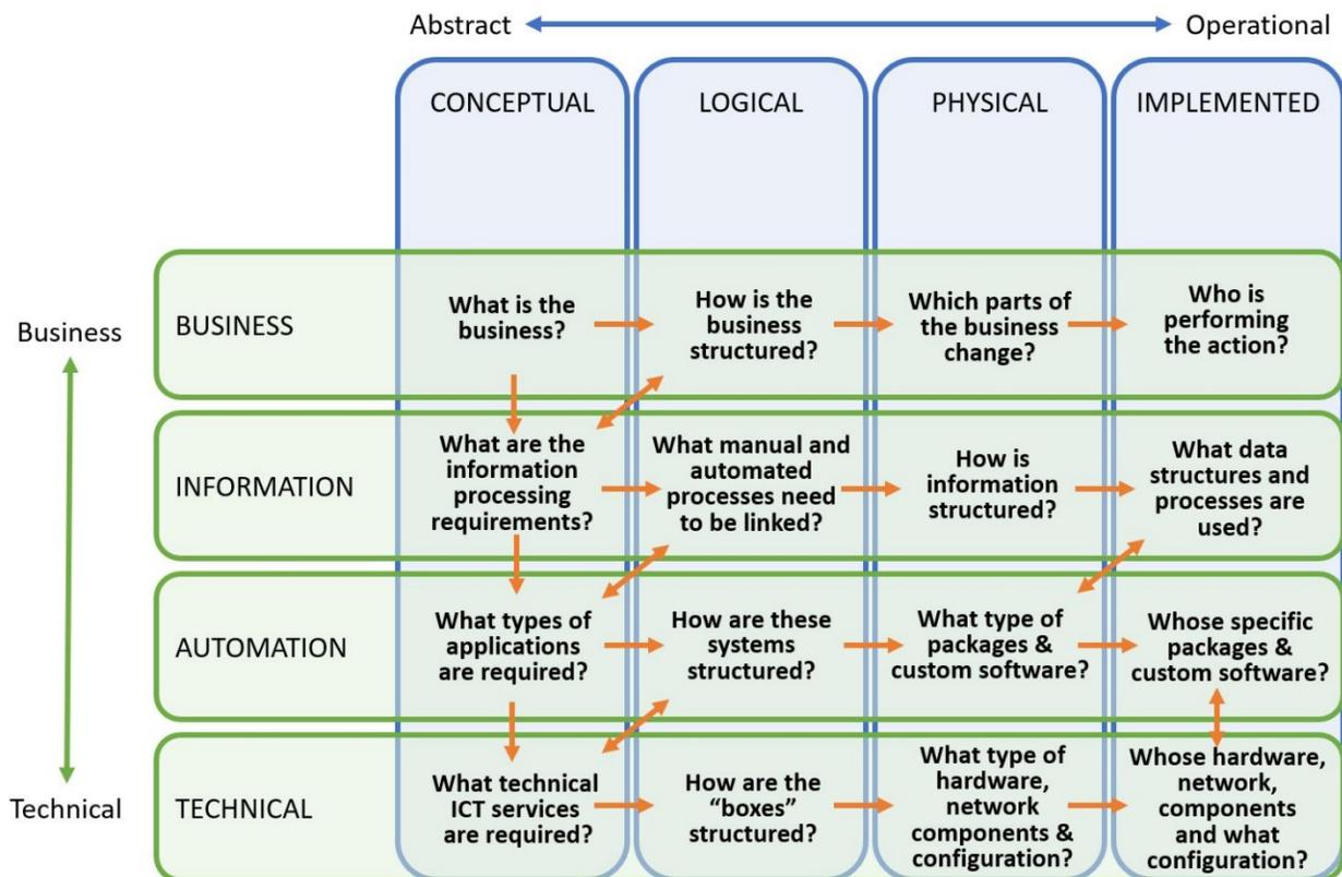
**Figure 9.** Architecture layers and iteration levels (Adapted from NIST Special Publication 1108r3 [NIST 2014]). ICT is information and communications technology.
