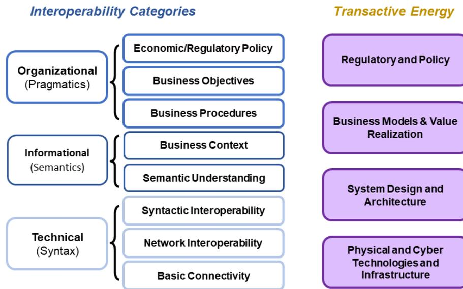
**Figure 6.** GWAC Stack with strata of transactive energy
