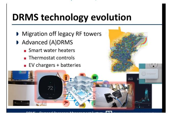
The warm water in the water heater is essentially a potential battery. The water can be heated a bit higher in advance of a planned outage to avoid running out of hot water during the outage.
